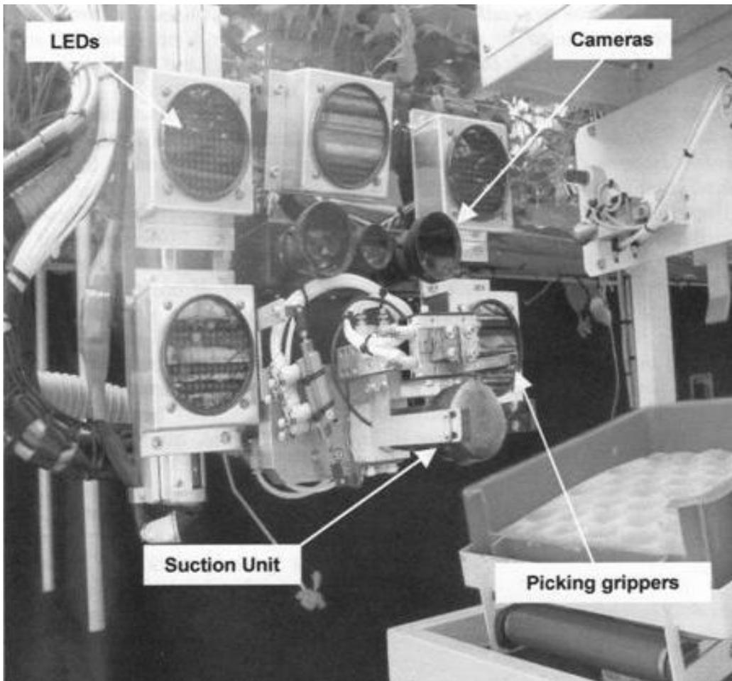
The cylindrical machine uses machine vision based around five LEDs and three cameras. The centre camera is used to detect the peduncle and the two
