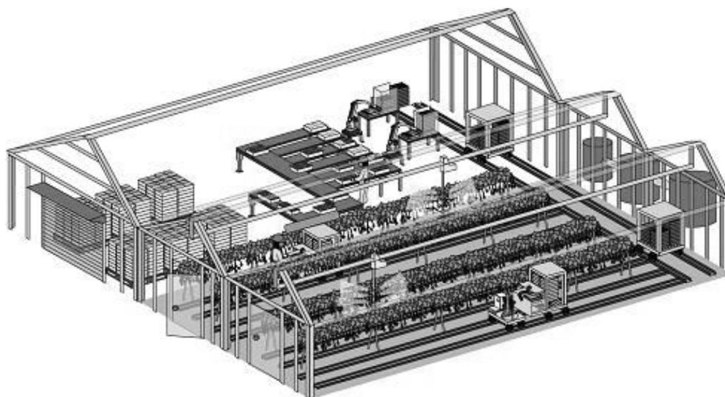
The robots are designed to work at night when shadow does not interfere with the machine vision. The robots travel on rails, are battery powered and work under LED lights. Cameras are used to identify the fruit and an algorithm calculates the proportion of the fruit that is white at the top to determine if the fruit should be picked.
